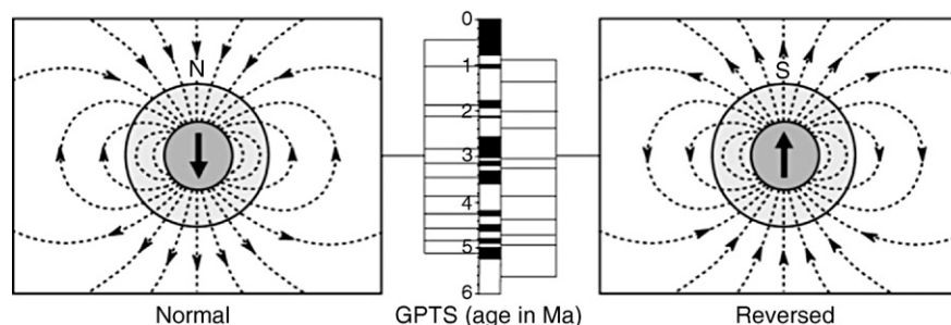
Figure D20 Schematic representation of the geomagnetic field of a geocentric axial dipole (“bar magnet”). During normal polarity of the field, the average magnetic north pole is at the geographic north pole, and a compass aligns along magnetic field lines, the inclination being positive (downward-directed) in the northern hemisphere and negative (upward-directed) in the southern hemisphere. Conversely, during reversed polarity, the compass needle points to the south, and the inclination is negative in the northern and positive in the southern hemisphere. In the GPTS, periods of normal and reversed polarity are represented by black and white colored intervals, respectively.
