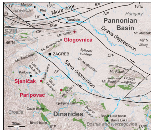
Fig. 2 The map shows the position of geographic and geologic features from the southern Pannonian Basin and adjoining Dinaride-Alpine fold-thrust belts that are referred to in the text. The white-shaded area represents Miocene to Pleistocene infill of the Pannonian Basin System starting with the Middle Miocene marine flooding. The dark green-shaded areas are Lower to Middle Miocene lacustrine deposits. Compiled after Fodor et al. (1999), Tomljenović and Csontos (2001), Jelen and Rifelj (2003), Pavelić et al. (2003), Saftić et al. (2003), Placer (2008), geologic maps of former Yugoslavia M 1:100,000 and M 1:500,000 and ESRI ArcGIS base maps. SZB Oligocene to Lower Miocene Slovenia-Zagorje Basin, PB Pannonian Basin, PF Periadriatic Fault, LF Lavantal Fault, SF Šoštanj Fault, CF Celje Fault, DoF Donat Fault, LjF Ljutomer Fault, BF Balaton Fault, NF Nagykanizsa Fault, SF Sava Fault, DrF Drava Fault
