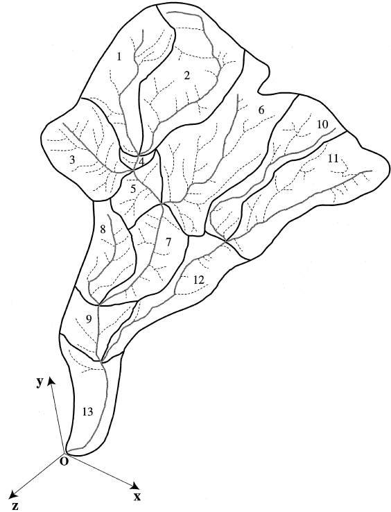
Fig. 3. A real world watershed subdivided into 13 REWs and the global reference system (Sabino Canyon, Santa Catalina Mountains, SE-Arizona, Reproduced from K. Beven and M.J. Kirkby, Channel Network Hydrology, Wiley.
