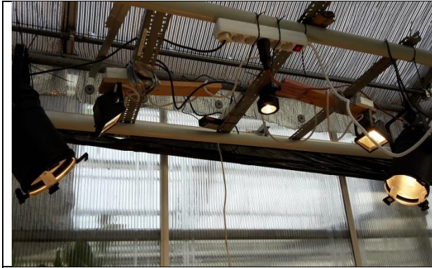
Lamp set 0: 3 halogen (50 and 2x300W) and 2 theatre lamps (1000 W).
