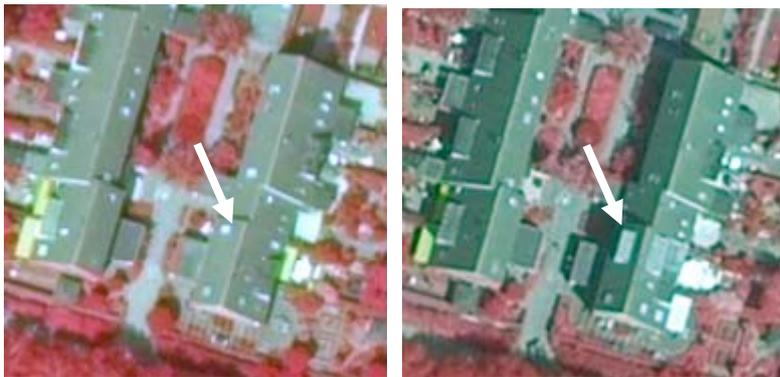
Figure 2: Roof vault added to existing house (left 2004, right 2005)
